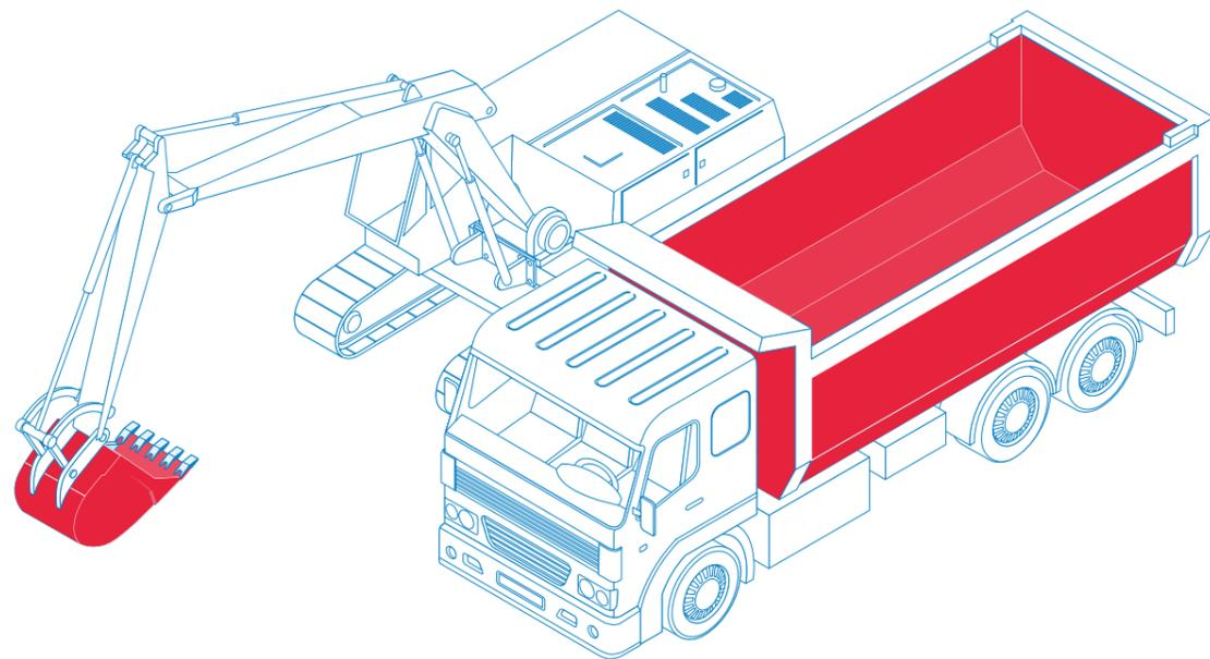
Valast 450 steel is harder than structural steel grades e.g. S355 and the abrasion resistance is up to 2.5 times greater.
